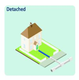
Detached properties, generally, drain on their own and, therefore, any pipework within the boundary is the responsibility of the homeowner. This may not be the case with modern detached properties built as part of a new development where drainage arrangements should be verified if necessary.
